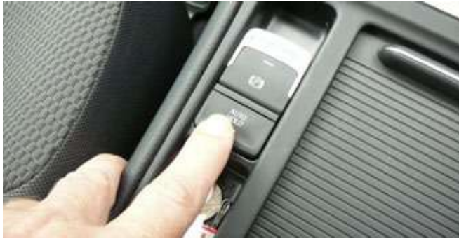
Figura 2.100. Control arranque pendiente
